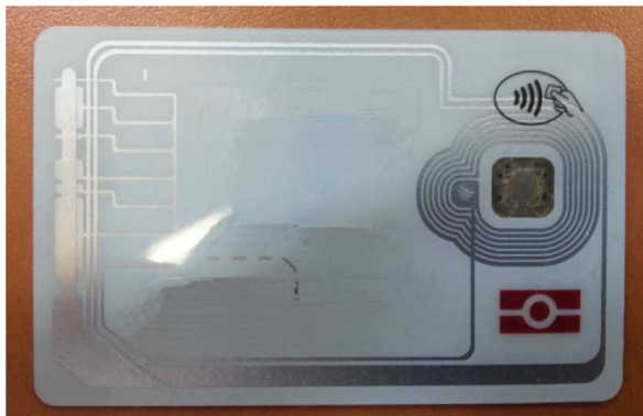
Fig. 5. Payment card IC contactless interface.
